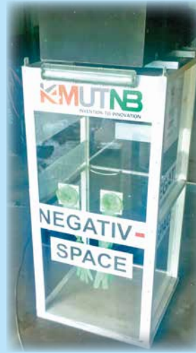
The positive pressure cabinet is designed for medical staff and the negative pressure cabinet is for patients infected with COVID-19.
